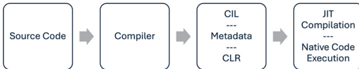
Figure 1.2: C# Program Compilation and Execution Process
