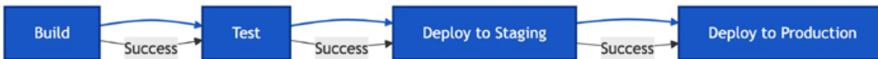
Figure 1.8: Jenkins Pipeline View, Showing Stages like Build, Test, and Deploy in a Web Interface
